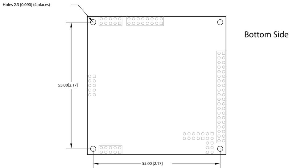
Mounting holes are equidistant from the center of the dspblok. These holes are 2.3mm in diameter, suitable for 2-56 or M2 screws. When 4.3mm height mating female connectors are used, the board will be 6.3mm (0.25 in) above the target board, therefore 0.250 standoffs may be used.
