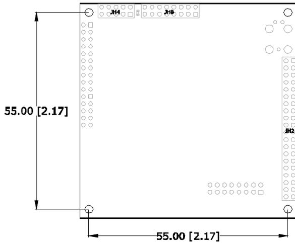
Mounting holes are equidistant from the center of the dspblok. These holes are 2.3mm in diameter, suitable for 2-56 or M2 screws. When 4.3mm height mating female connectors are used, the board will be 6.3mm (0.25 in) above the target board, therefore 0.250 standoffs may be used.
