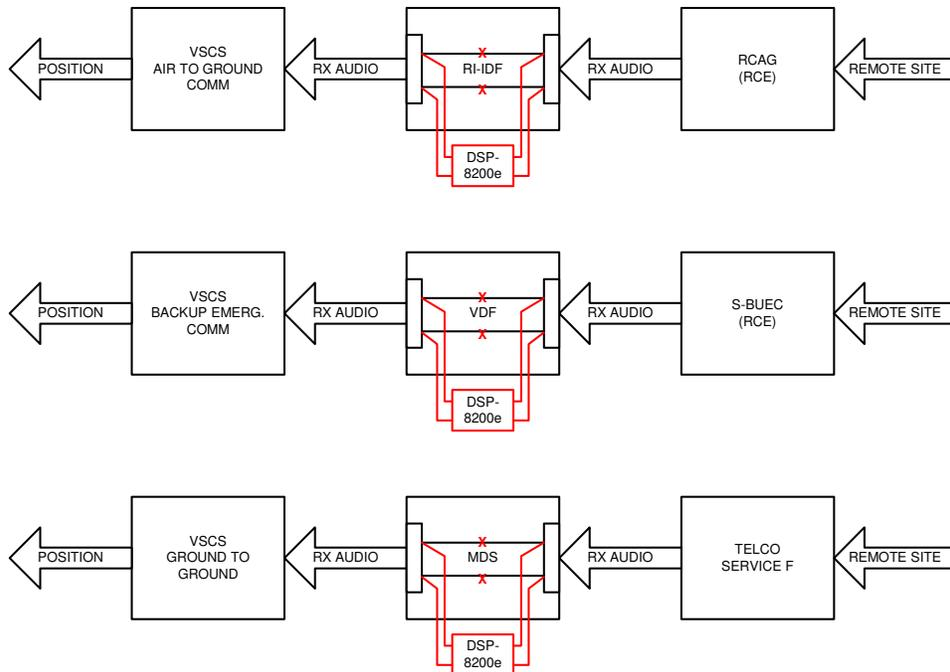
The DSP-8200e is useful in many FAA applications. Each module can be configured for tone suppression or broadband noise reduction.
