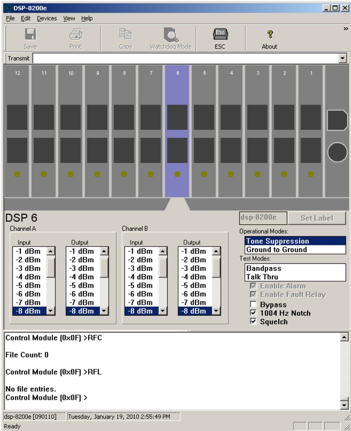
Modules can be set up globally or individually. If you want to set up all modules globally, you click on the Control Module in the DSP-8200e graphic. This will cause all the modules to change to blue. If all modules are set to the same parameters, then the selections will also be highlighted.
