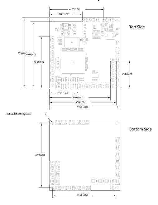
Mounting holes are equidistant from the center of the dspblok. These holes are 2.3mm in diameter, suitable for 2-56 or M2 screws. When 4.3mm height mating female connectors are used, the board will be 6.3mm (0.25 in) above the target board, therefore 0.250 standoffs may be used.
