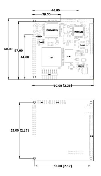
Mounting holes are equidistant from the center of the dspblok. These holes are 2.3mm in diameter, suitable for 2-56 or M2 screws. When 4.3mm height mating female connectors are used, the board will be 6.3mm (0.25 in) above the target board, therefore 0.250 standoffs may be used.
