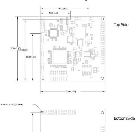
Mounting holes are equidistant from the center of the dspblok. These holes are 2.3mm in diameter, suitable for 2-56 or M2 screws. When 4.3mm height mating female connectors are used, the board will be 6.3mm (0.25 in) above the target board, therefore 0.250 standoffs may be used.
