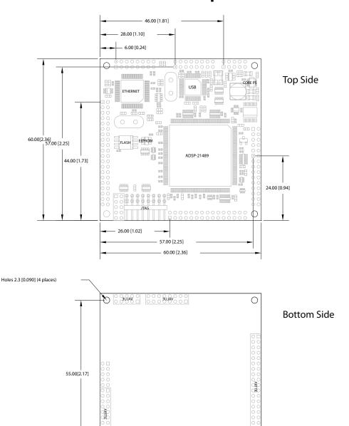
Mounting holes are equidistant from the center of the dspblok. These holes are 2.3mm in diameter, suitable for 2-56 or M2 screws. When 4.3mm height mating female connectors are used, the board will be 6.3mm (0.25 in) above the target board, therefore 0.250 standoffs may be used.
