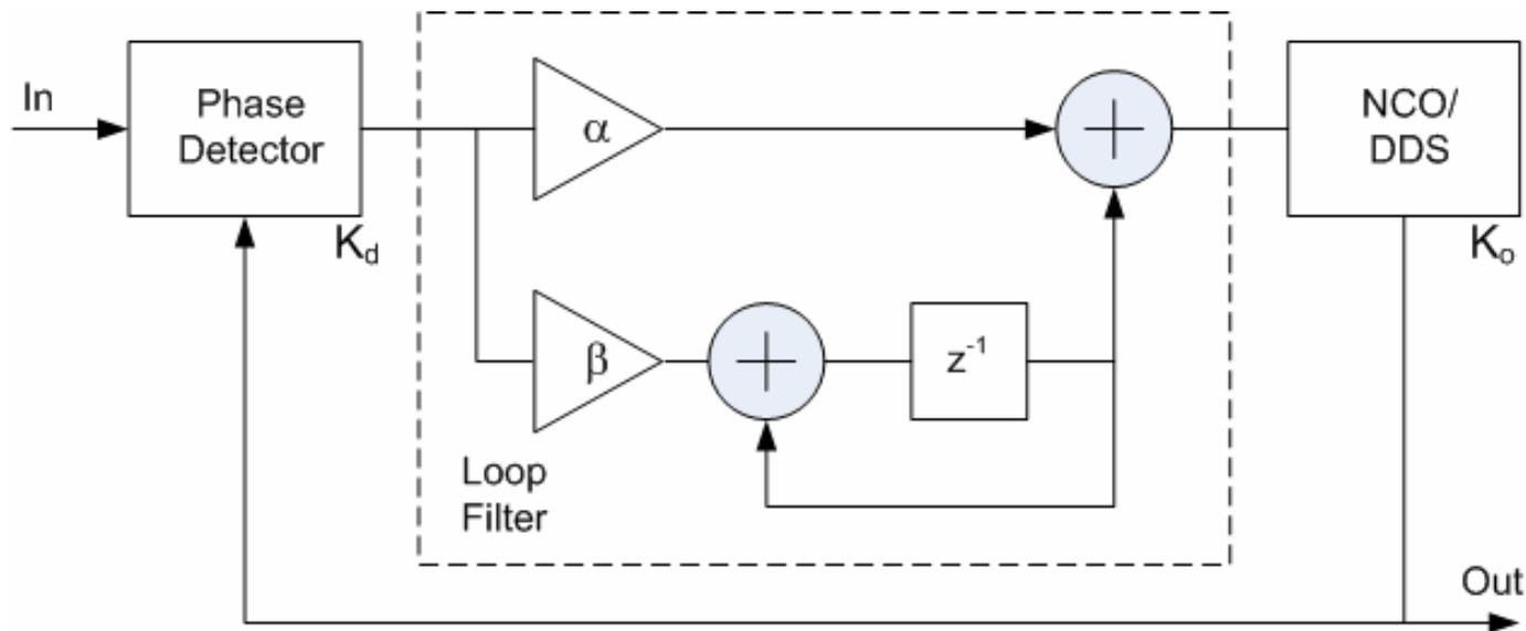
The input multiplier has been replaced with a suitable digital phase detector, and the VCO has been replaced with an NCO/DDS. The next step is analyzing these components and their characterizing gains  $K_o$  and  $K_d$ .
