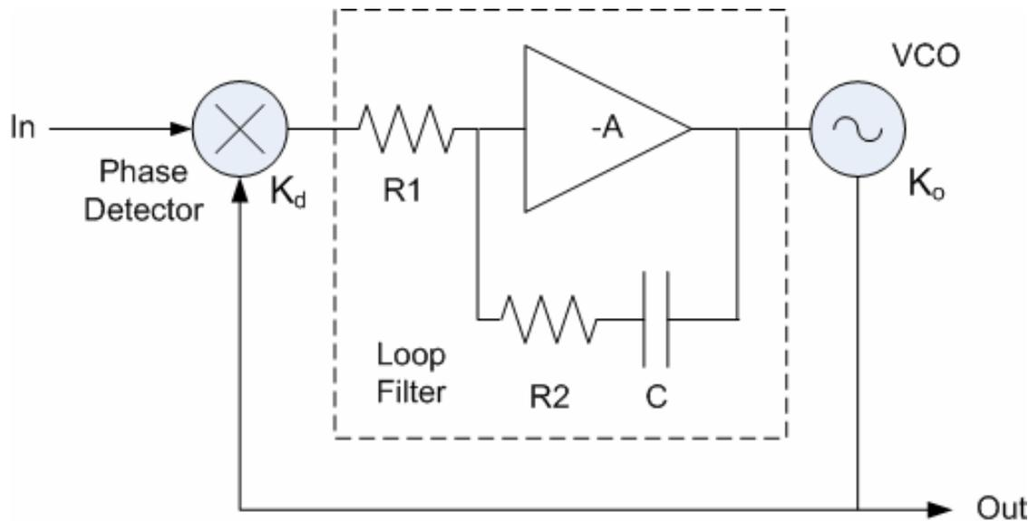
The basic loop components are the Phase Detector, Loop Filter, and VCO.
