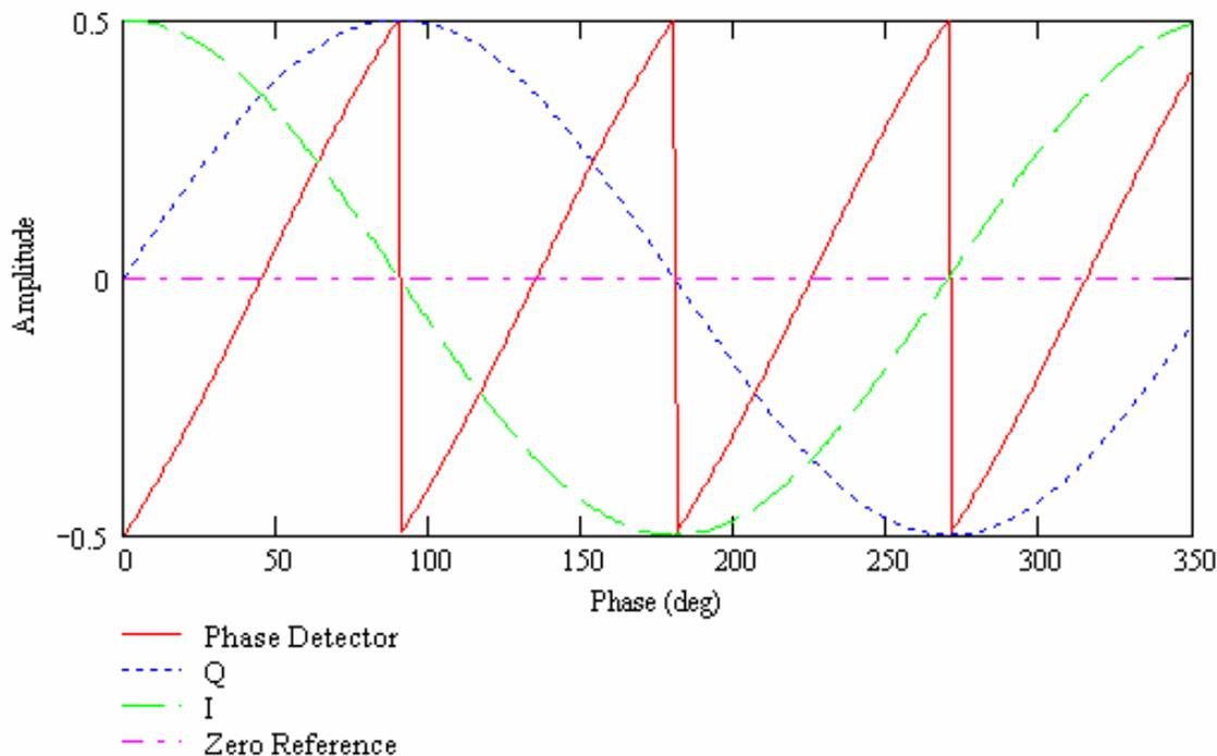
So for this detector, where the maximum output value is 1.0,  $K_d = 1/\pi$  MSB/rad. i.e., a set MSB = 1 radian.
