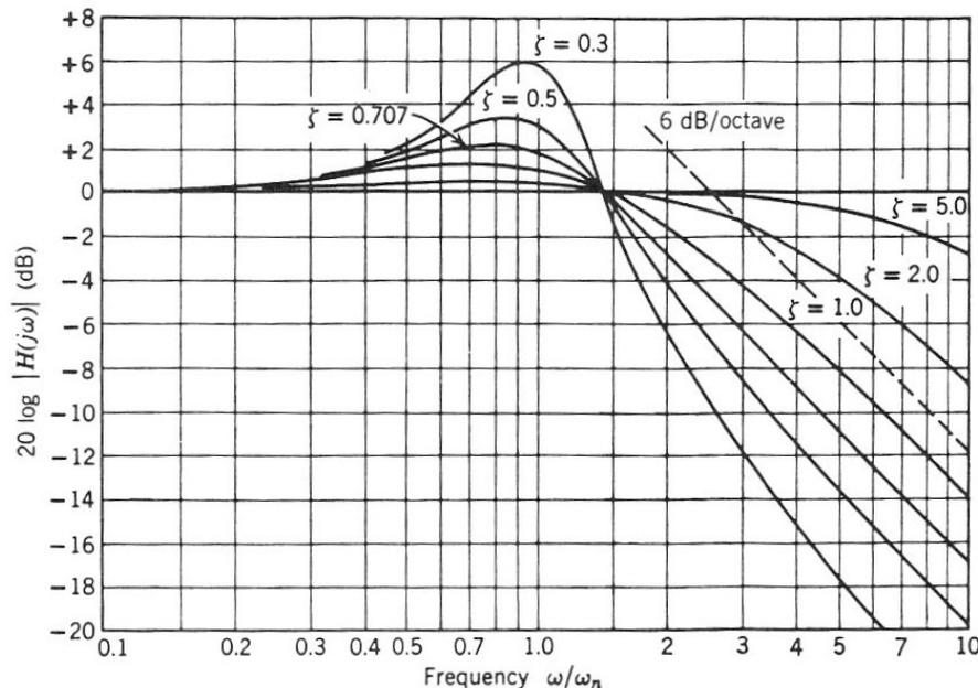
Figure 2.3 Frequency response of a high-gain second-order loop.
